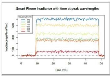
While the spectral stability of the flash appeared quite high, we were curious to look at it more closely. A color temperature plot over time showed a slight upward trend in color temperature, roughly 500 K over 15 ms. This was supported by high color consistency as shown in the very stable chromaticity diagram plot. With zooming, we would see on the plot that flash color varied by <0.02 in x and y over the lifetime of the three flashes measured.
