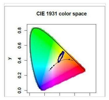
The black line on the chromaticity diagram indicates standard blackbody color values (the actual definition of a color temperature), with the black dots indicating color temperatures of 2000 K, 4000 K and so on. The dark blue line tracing the yellow portion of the chromaticity diagram shows the color value of the fluorescent lights as they cycle through the 50 Hz AC oscillations – a fairly wide swing in perceived color!
