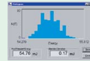
Distribution of the output energy per pulse for 500 consecutive shots. Range of histogram ± 1% of mean value. Standard deviation -0.3%.
