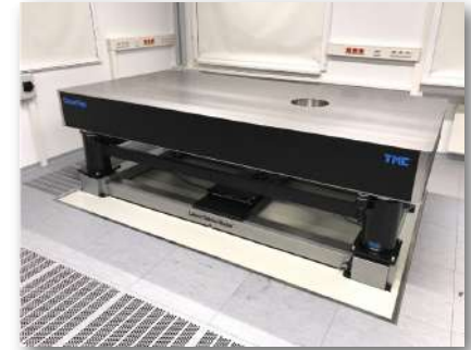
Figure 7. Example of a combined system - active isolation on the bottom and passive on the top
